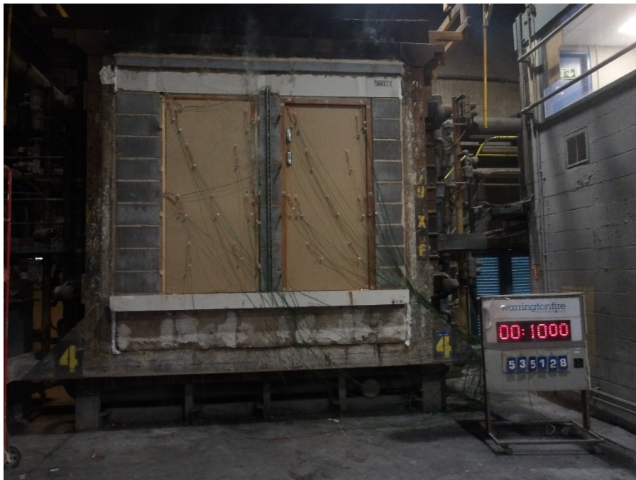
Figure 18 Unexposed face of the specimens after 10 minutes of testing.
