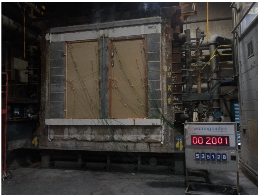
Figure 19 Unexposed face of the specimens after 20 minutes of testing.
