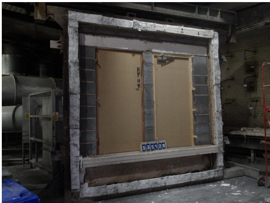
Figure 17 Exposed face of the specimen before the start of the test
