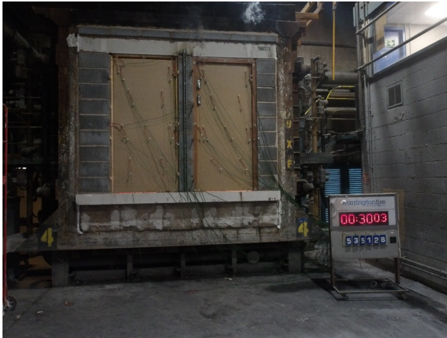
Figure 20 Unexposed face of the specimens after 30 minutes of testing.
