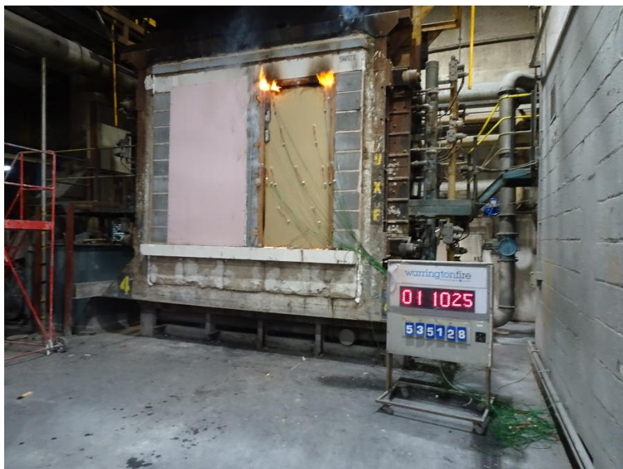
Figure 25 Unexposed face of Doorset B after 70 minutes of testing prior
