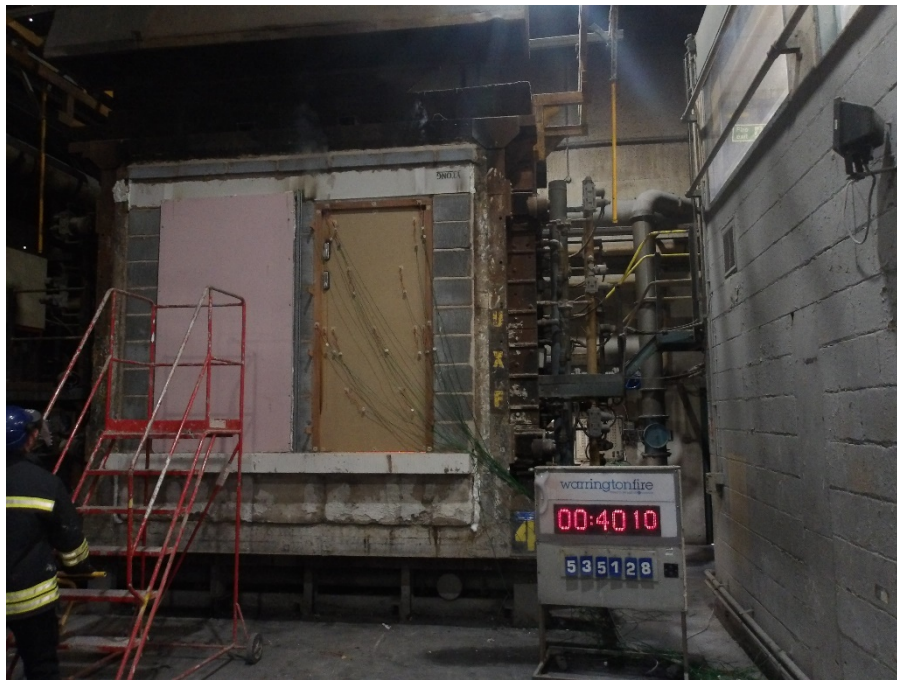
Figure 22 Unexposed face of the Doorset B after 40 minutes of testing
