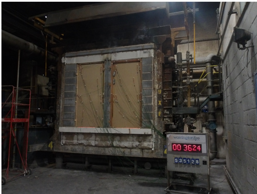
Figure 21 Unexposed face of the specimens after 36 minutes of testing prior to blanking off Doorset A.
