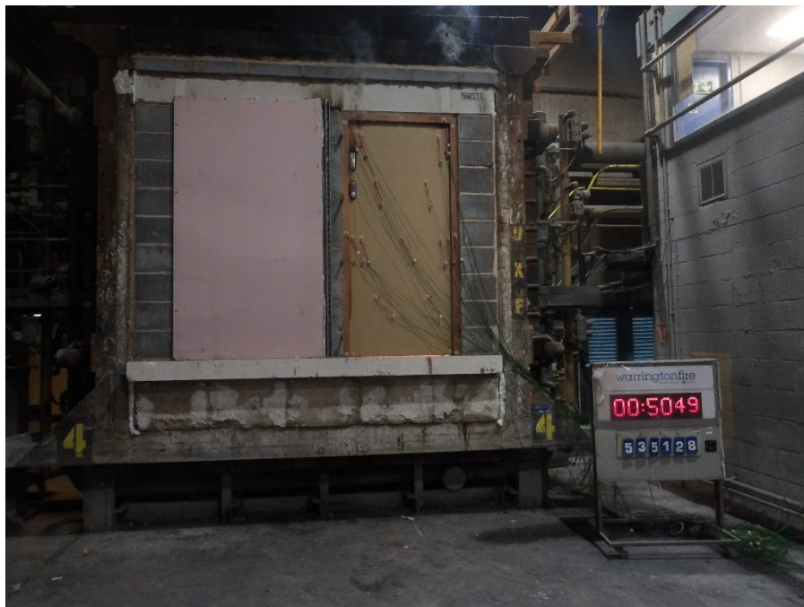
Figure 23 Unexposed face of the Doorset B after 50 minutes of testing
