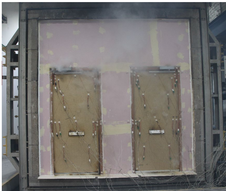
Figure 22 - The unexposed surface of the test construction after a test duration of 50 minutes
