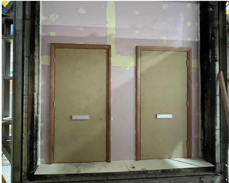
Figure 15 – The exposed surface of the test construction prior to commencement of the test
