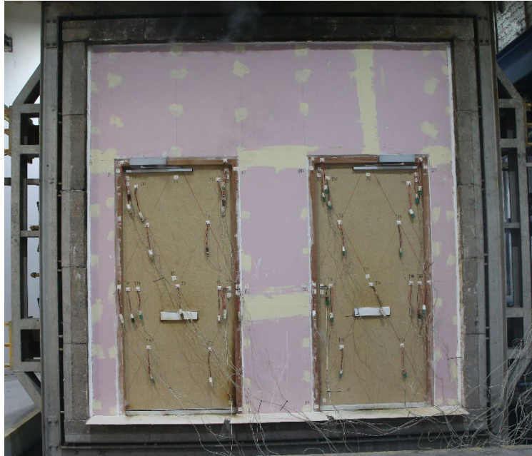
Figure 19 - The unexposed surface of the test construction after a test duration of 20 minutes
