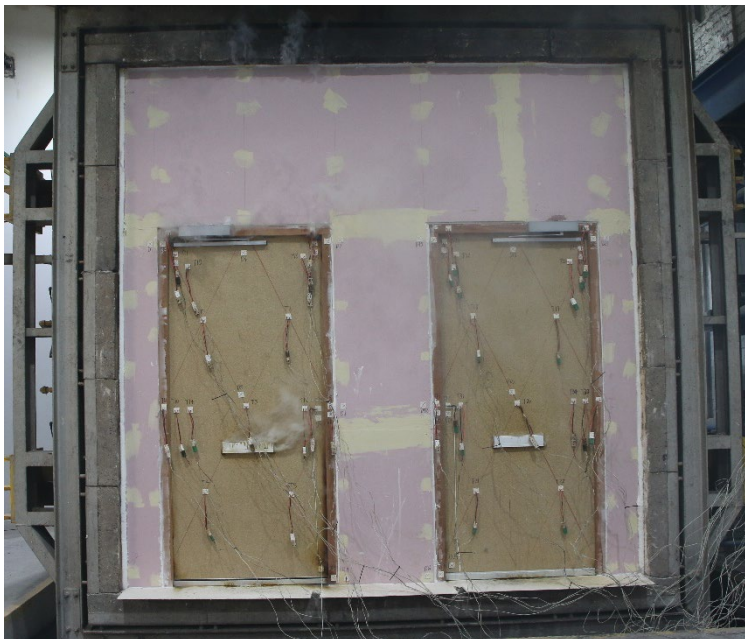
Figure 20 - The unexposed surface of the test construction after a test duration of 30 minutes
