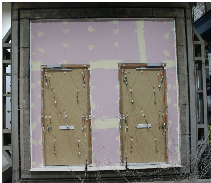
Figure 16 - The unexposed surface of the test construction prior to the commencement of the test
