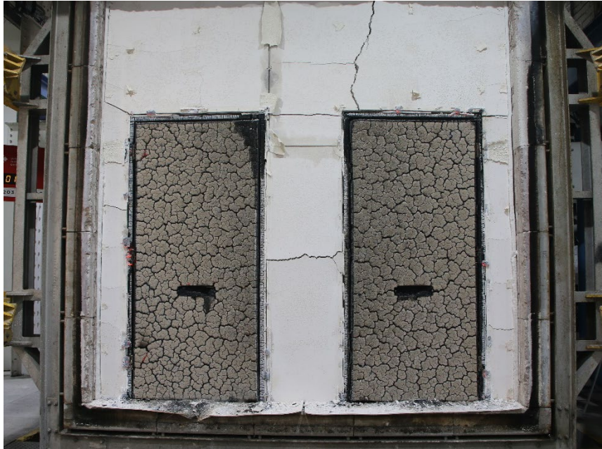
Figure 25 - The exposed surface of the test construction after the test was discontinued
