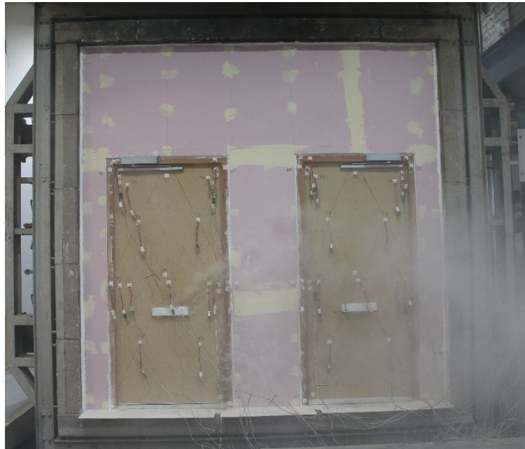
Figure 17 - The unexposed surface of the test construction after a test duration of 6 minutes
