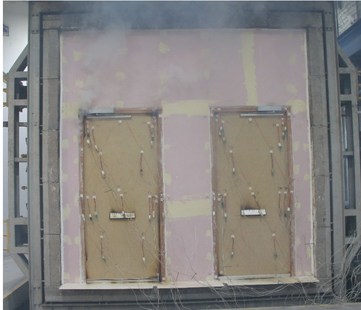
Figure 23 - The unexposed surface of the test construction after a test duration of 55 minutes
