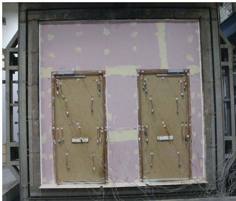
Figure 18 - The unexposed surface of the test construction after a test duration of 10 minutes
