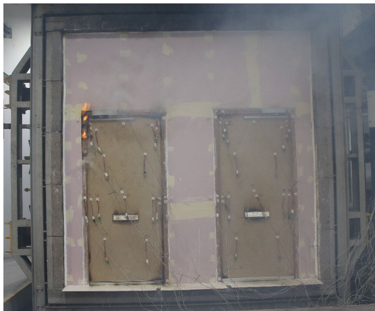
Figure 24 - The unexposed surface of the test construction after a test duration of 68 minutes
