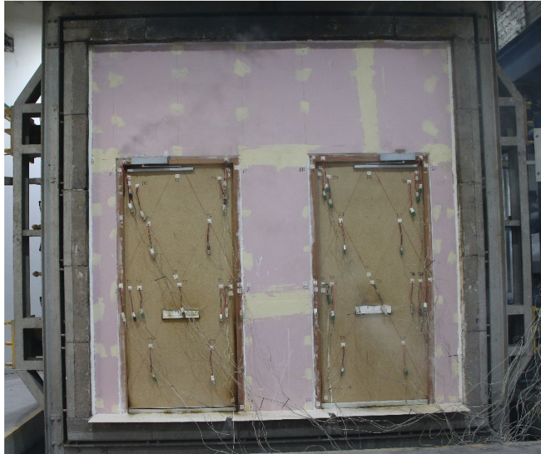
Figure 21 - The unexposed surface of the test construction after a test duration of 40 minutes
